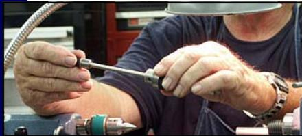
The rod blank can be held with a pen mandrel chuck end
